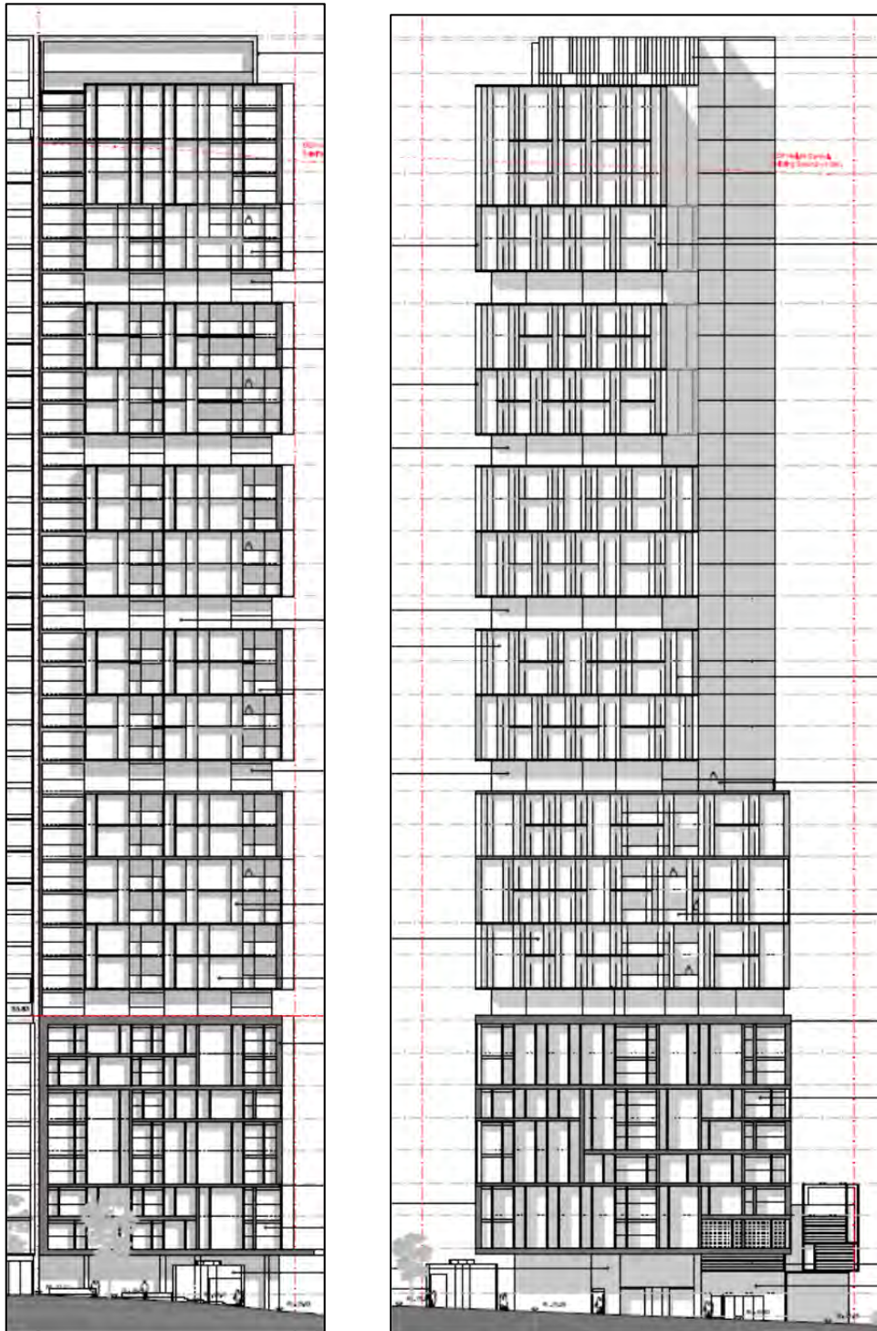
Figures 14 and 15: Elevation drawings of the northern (Liverpool Street) elevation (left) and the western (Elizabeth Street) elevation (right). Both elevations illustrate the amended scheme
