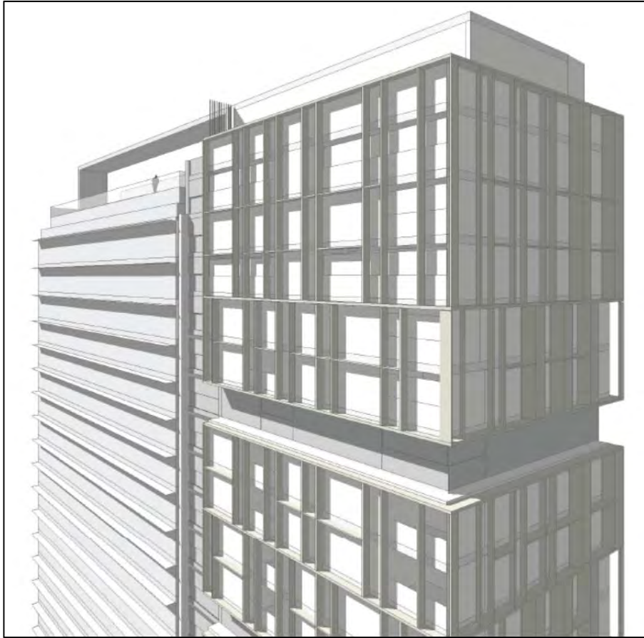
Figure 38: View of the proposed parapet/wind mitigation screen around the perimeter of the penthouse roof terraces
