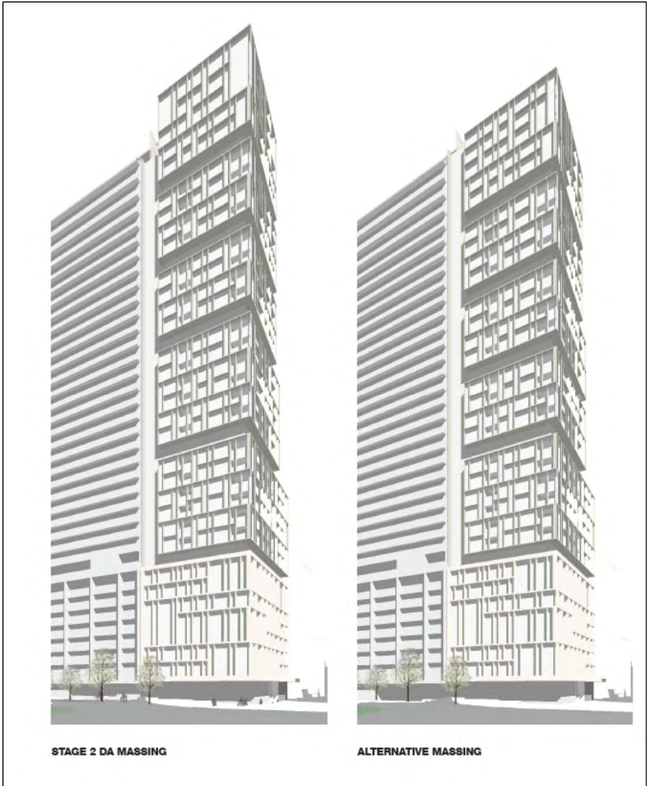
Figures 27 and 28: The scheme as originally lodged (left) and, as modified with the upper two levels setback (right), as viewed from Elizabeth Street looking south
